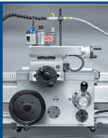
Electromechanical stop for cutting right-hand and left-hand threads.
