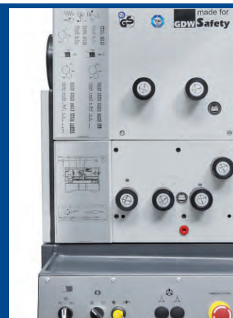
Spindle housing with safety interlock for high torques (LZ 400 V).
